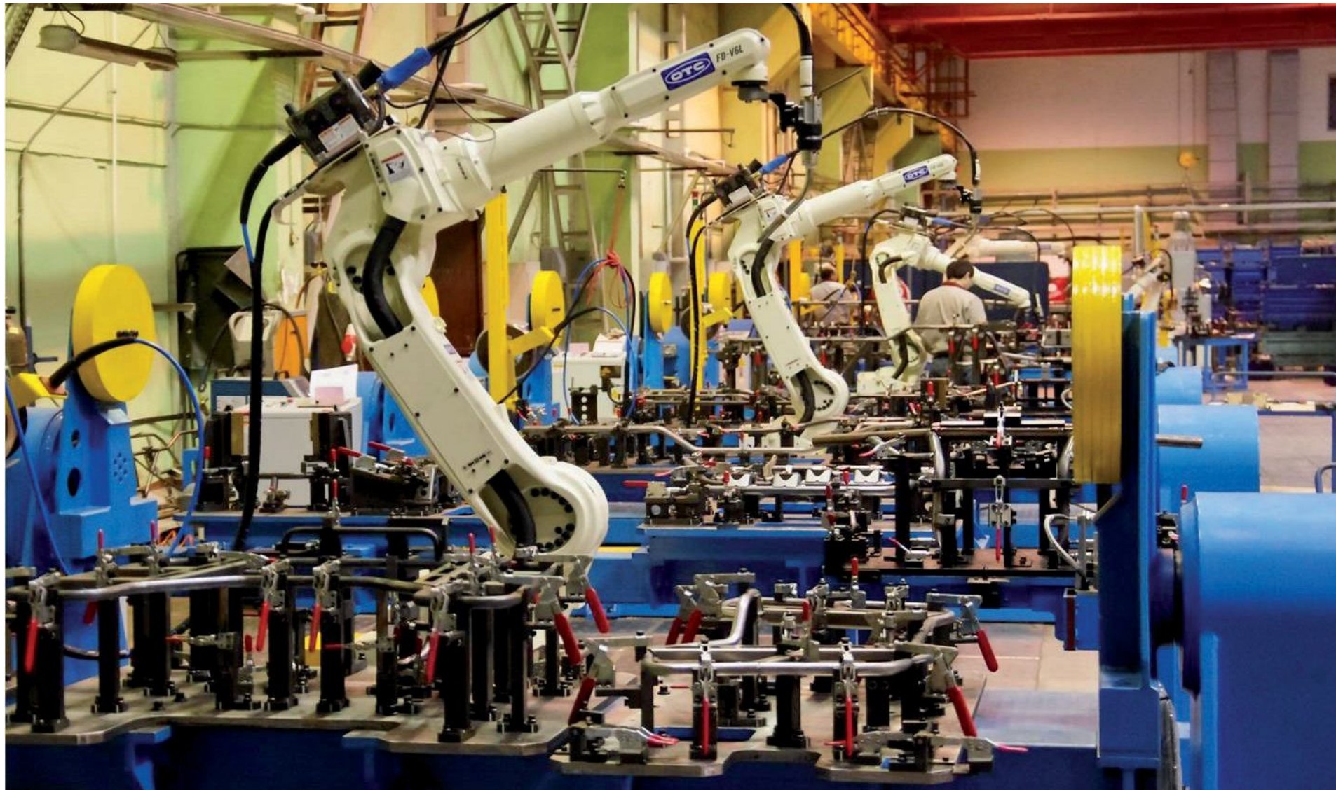
Robotic welding area
